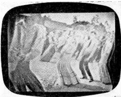
Fig. 6—A single ripple in picture, with straight raster edges and no hum bar indicates hum in the horizontal sync or a-f-c circuits.
